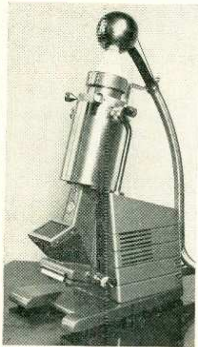
FIG. 5—Microscope column with protective hood removed
