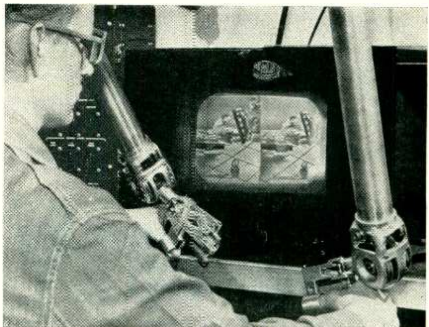
Single-tube stereo-television viewer monitoring the pouring of a liquid by a mechanical master-slave manipulator
