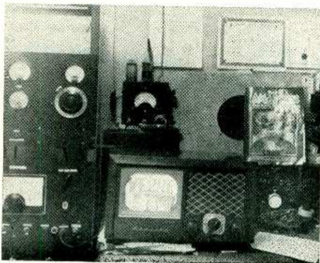
Equipment used in recent amateur tv transmissions showing the r-f portion of the transmitter, monitoring set, and phototube and video amplifier chassis facing test transparency on face of the transmitting crt
