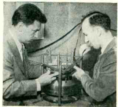
Accurate measurements of resonant frequency of microwave cavity permit determination of the speed of light with 0.0002-percent accuracy
